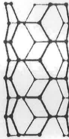
Figure 8. (a)The C 60 fullerene molecule, where there are 12 pentagons necessary to produce the spherical configuration. Carbon Nano-tube of arm chair type (b) and of zigzag type(c).It is not necessary to introduce pentagons for producing nano-tubes as they have zero curvature.[Pachos (2009)]
